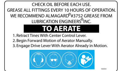
Fig. 4 LABEL AERATING INST PL
