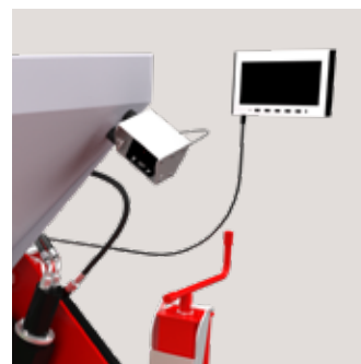
Camera to monitor the filling area.
