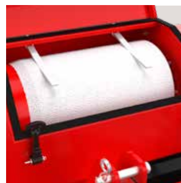
Vacuum system with dust bag to collect fines and dust.
