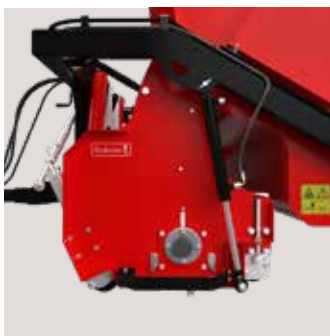
Floating head to manage undulations.
