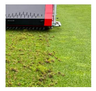
As the Scarivator loosens the top layer, it addresses naturally occurring hardpan in the soil profile. This hardpan is a concrete-like layer that can hinder proper root development and water absorption. The Scarivator etches away at this hardpan, leveling the surface and ensuring that the Turf-Stripper can perform optimally without damaging the backing, particularly on hybrid carpets.
